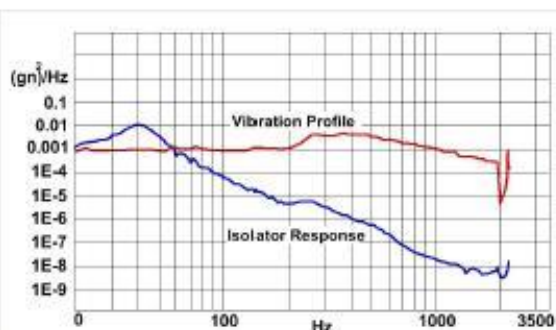
Figure 5: Vibration Profile and Isolator Response with a 40 Hz Resonance
