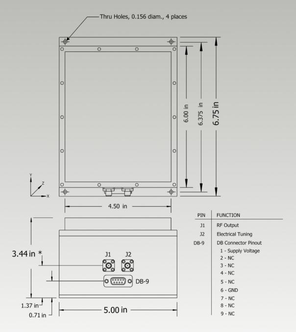
\* Internally vibration isolated version shown. Case height will be 2.5" on non-isolated models.
